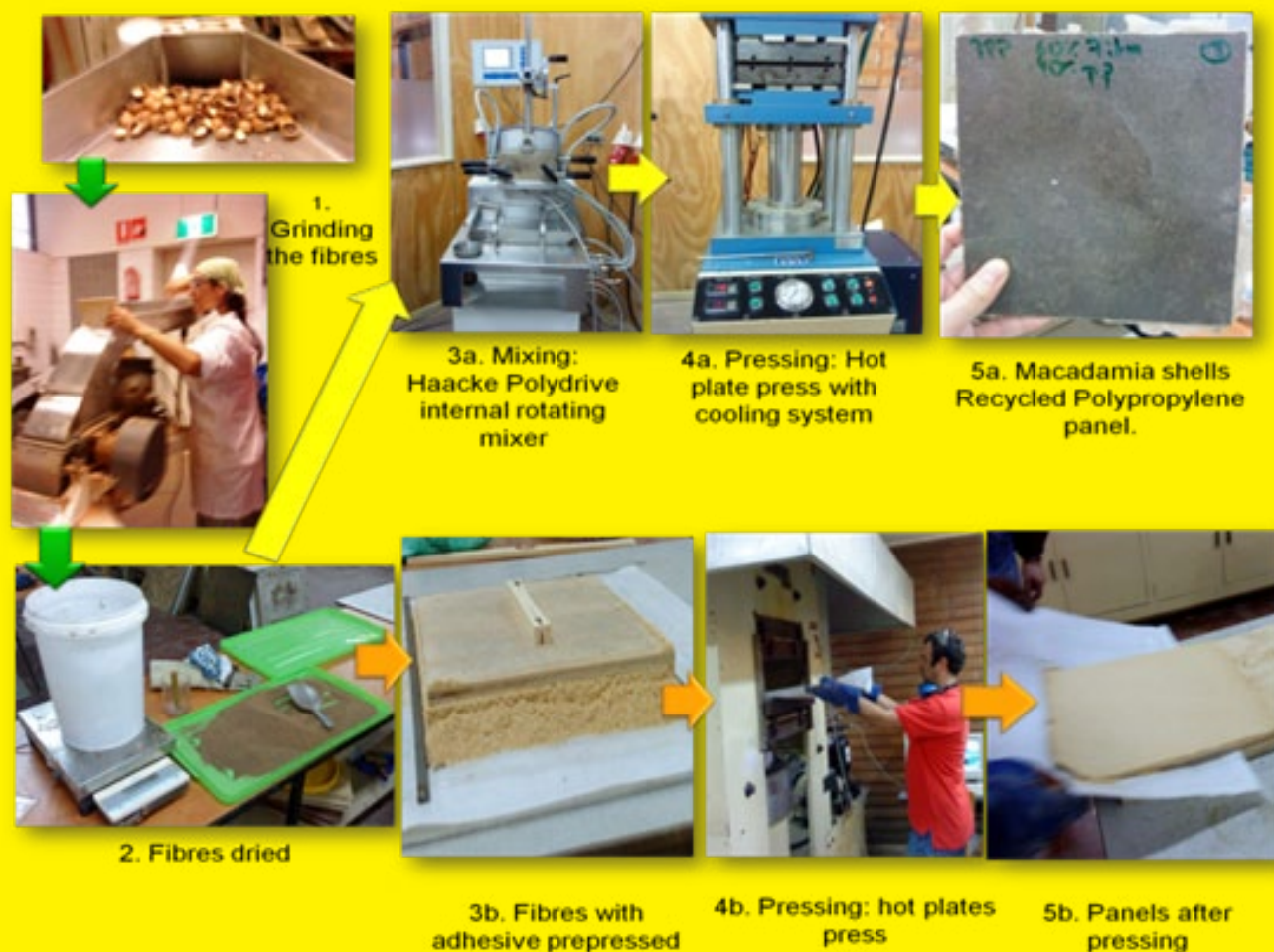
Figure 4 Schematic diagram of production process of the panels
