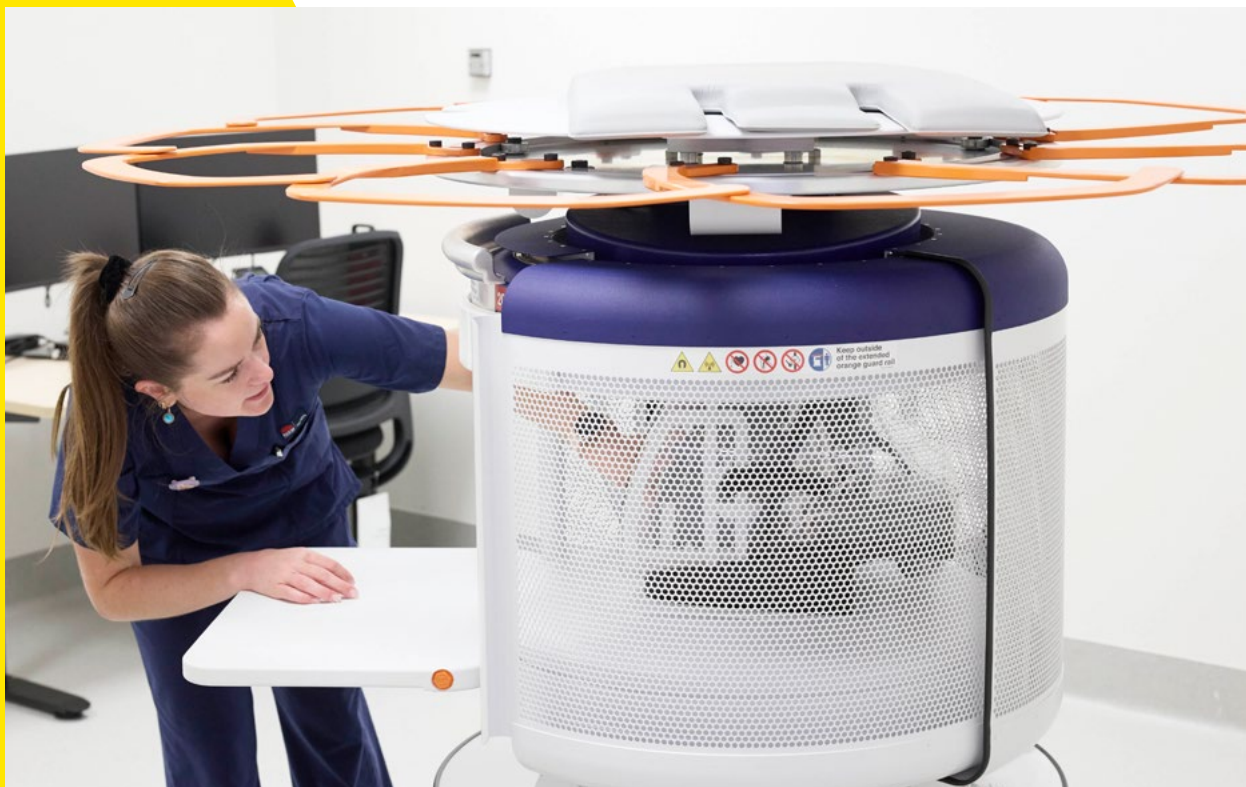
Research manager Julia Hennessey uses a new Hyperfine low-field MRI in UNSW's Integrated Acute Services Building. The portable MRI can move to patients' bedsides at the point of care, plug into a standard electrical outlet and acquire critical neuroimages within minutes.
